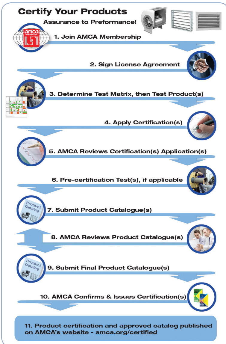
Figure 4. The 11 steps manufacturers must follow for their products to be licensed to bear the AMCA CRP seal.
