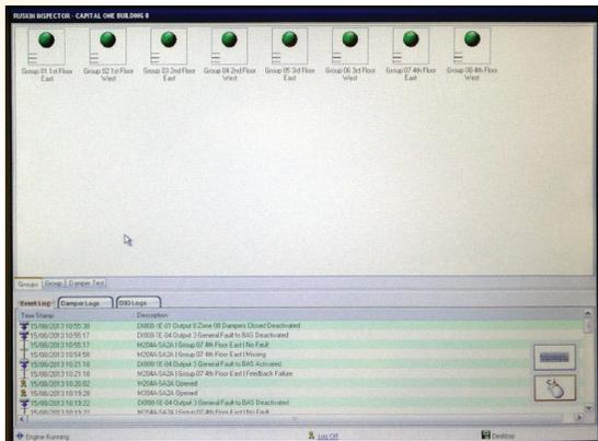
**Figure 3.** The screenshot shows the damper in the system, and the green dot indicates normal status. Three parallel lines indicate the damper is in the open position. There is an event log on bottom. Image courtesy of Ruskin
