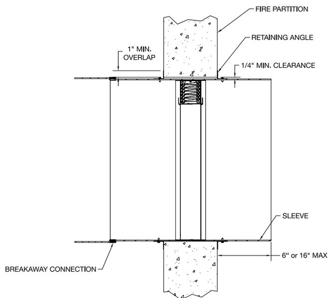
**Figure 2:** Typical fire damper installation, based on AMCA 503, *Fire, Ceiling (Radiation), Smoke and Fire/Smoke Dampers Application Manual*. Image courtesy of Ruskin.
