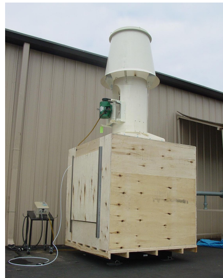
Induced Flow Fan mounted on plenum with side inlet
