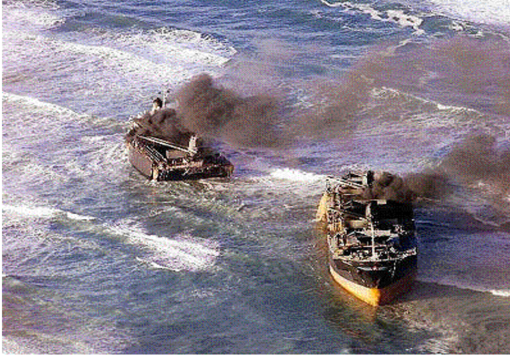
Figure 2 Tanker fatigue failure
