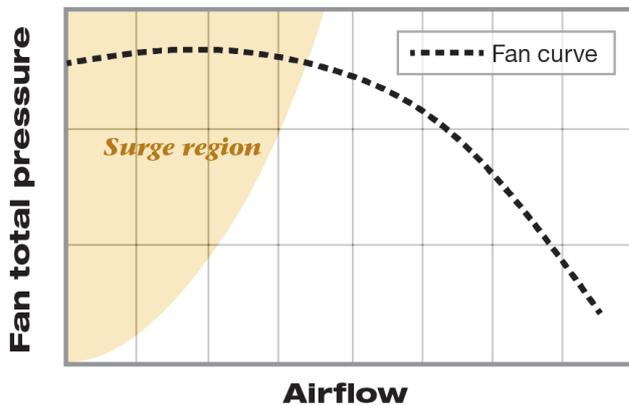
Figure 5: Typical Fan Curve Showing Surge Region
