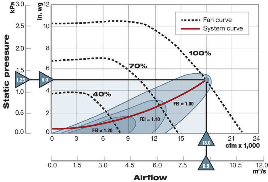
Figure 4: FEI Bubble Curve for 22-in. (565-mm) Backward-Inclined Fan Showing Compliance at all Three Duty Points of Interest
