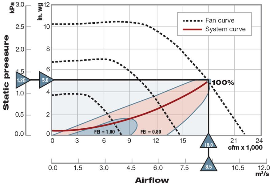
**Figure 3: FEI Bubble Curve for 18-in. (464-mm) Backward-Inclined Fan Showing Compliance at Low Flow Rates, but not at the Peak Design Condition**
