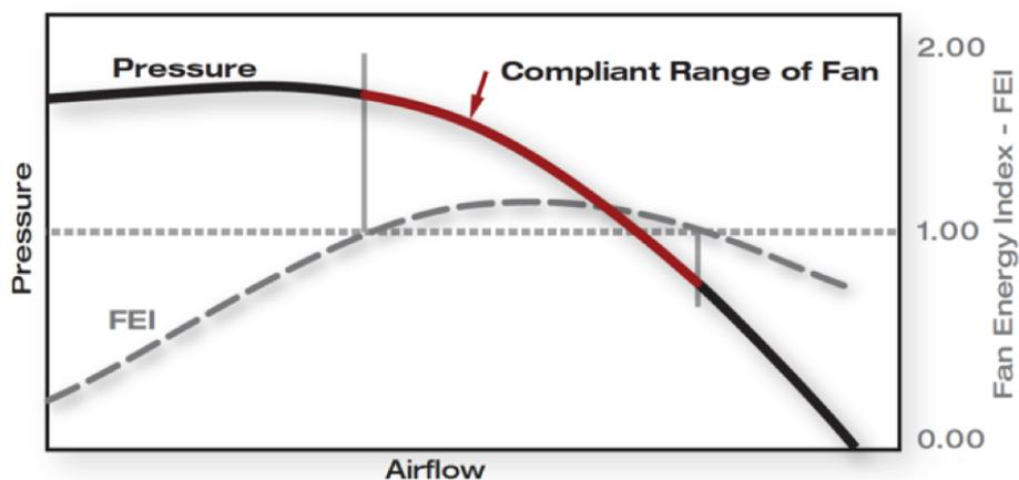
**Figure 1: Compliant Range of Duty Points for a Constant-Speed Fan for a Minimum FEI of 1.00**
