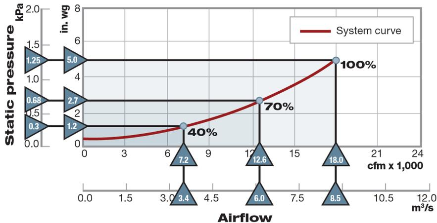
**Figure 2: Operating Points in a Typical VAV System**
