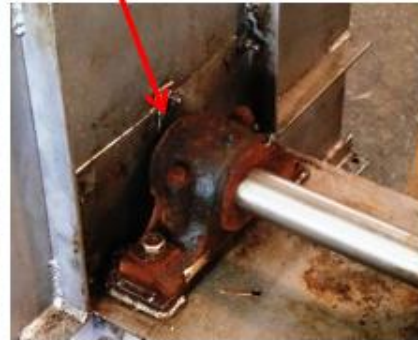
Leakage through seal causing bearing damage
