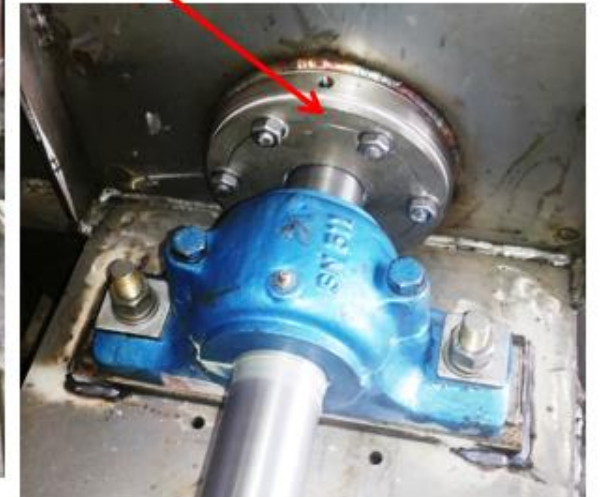
Labyrinth Seal with positive compressed air supply
