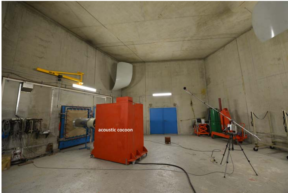
Reverberant room method (inlet noise in category B configuration)
