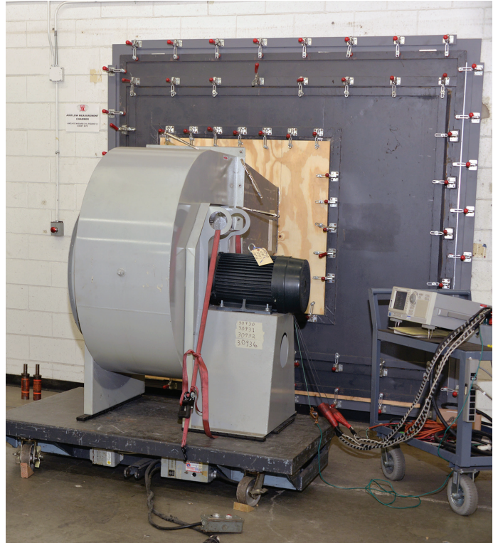
Fan air-performance (above) and damper leakage testing (below) at AMCA International headquarters laboratory.
