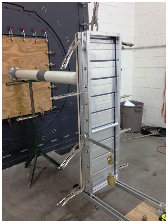
Fan air-performance (above) and damper leakage testing (below) at AMCA International headquarters laboratory.
