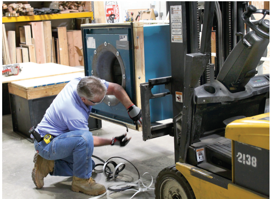
A fan being prepared for testing at the AMCA International headquarters laboratory.
