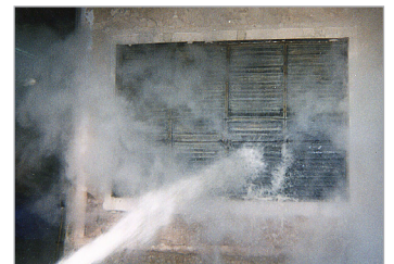
A fire/smoke damper undergoing UL hose stream testing. Image courtesy of Nailor Industries
