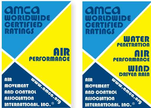
Figure 1. Example AMCA CRP seals for fans and dampers (left) and louvers (right). Note that multiple certifications can be combined into one label.
