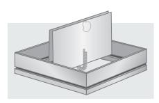
Figure 4. Example UL 555C-classified ceiling damper.
