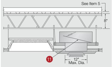
**11. Damper** — No. 13 MSG galv steel, 14 by 14 in. Protected on both surfaces with 1/16 in. ceramic fiber paper and held open with a Fusible Link. (Bearing the UL Listing Mark). Damper to overlap duct outlet 1 in. min.
