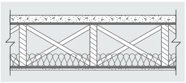
Figure 3. Example floor/ceiling assembly in which installation of ceiling dampers is prohibited.
