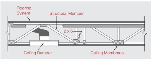
Figure 1. Example fire-rated floor/ceiling assembly.
