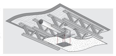
Figure 7. Example combustible floor/ceiling assembly.
