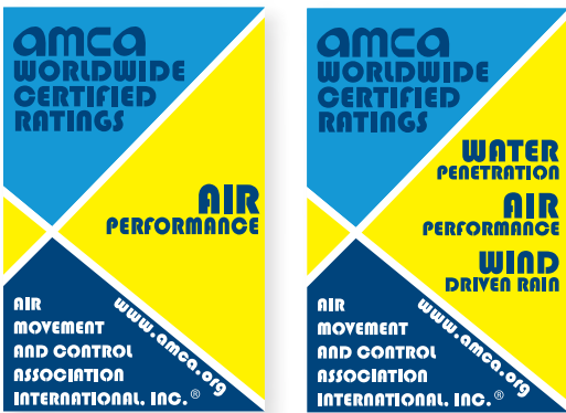
FIGURE 1. AMCA CRP seals for fans and dampers (left) and louvers (right). Note multiple certifications can be combined on one label.
