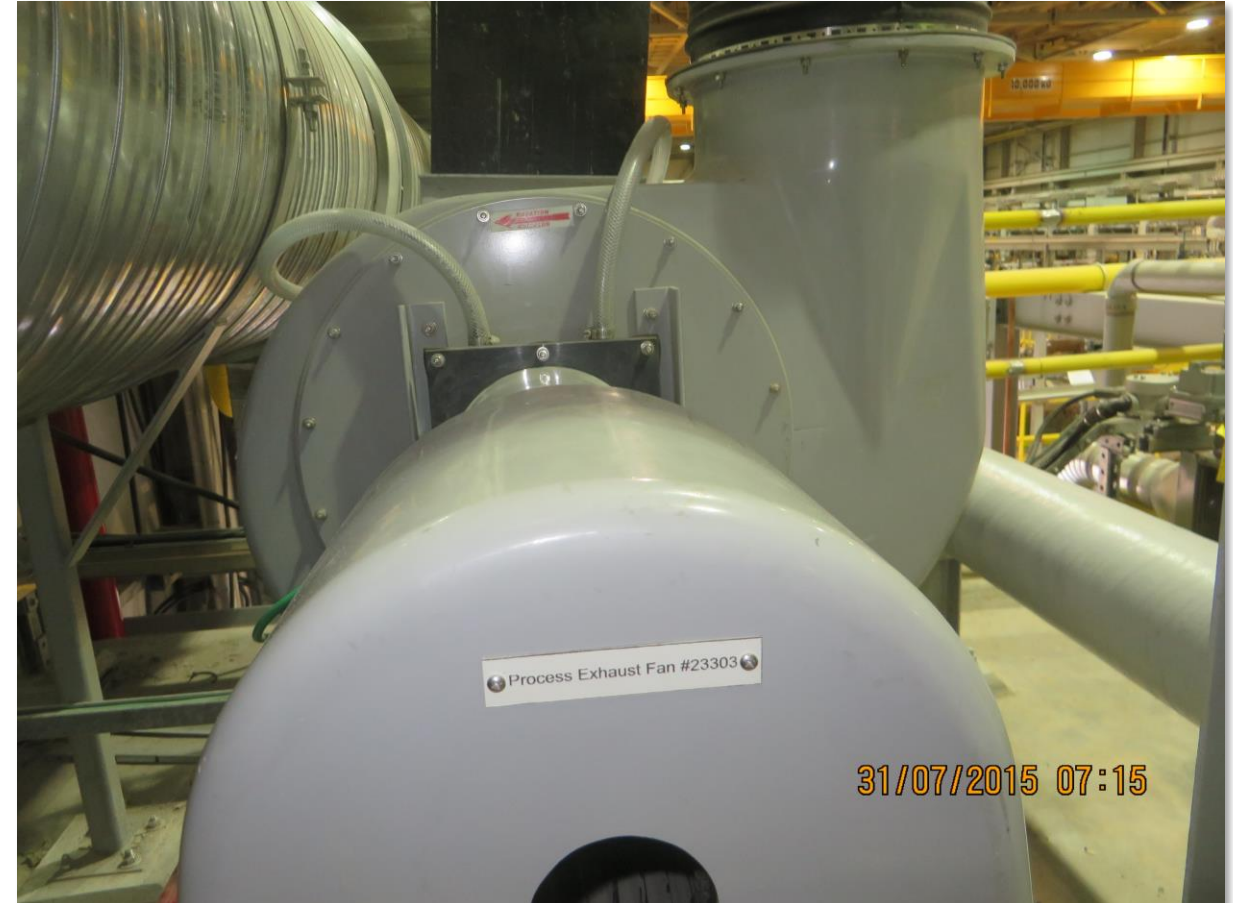
FRP fan installed in 1996 at Minatco (currently Orano) for their uranium processing McClean Lake Mill
