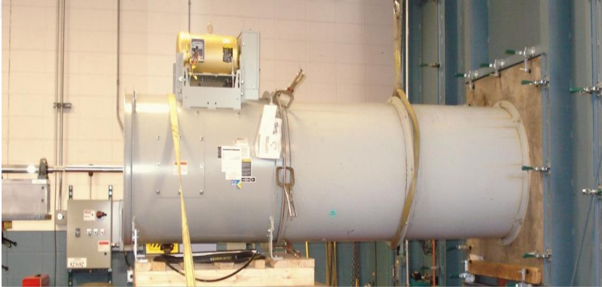
AMCA 210/ASHRAE 51 Test, Figure 12, Installation Type B Extended fan shaft allows Dynamometer or Motor driven
