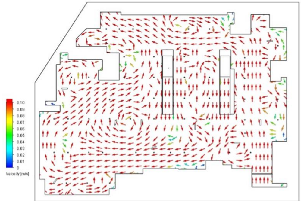
Figure 2: Velocity Vectors at 1.8m Level 0
