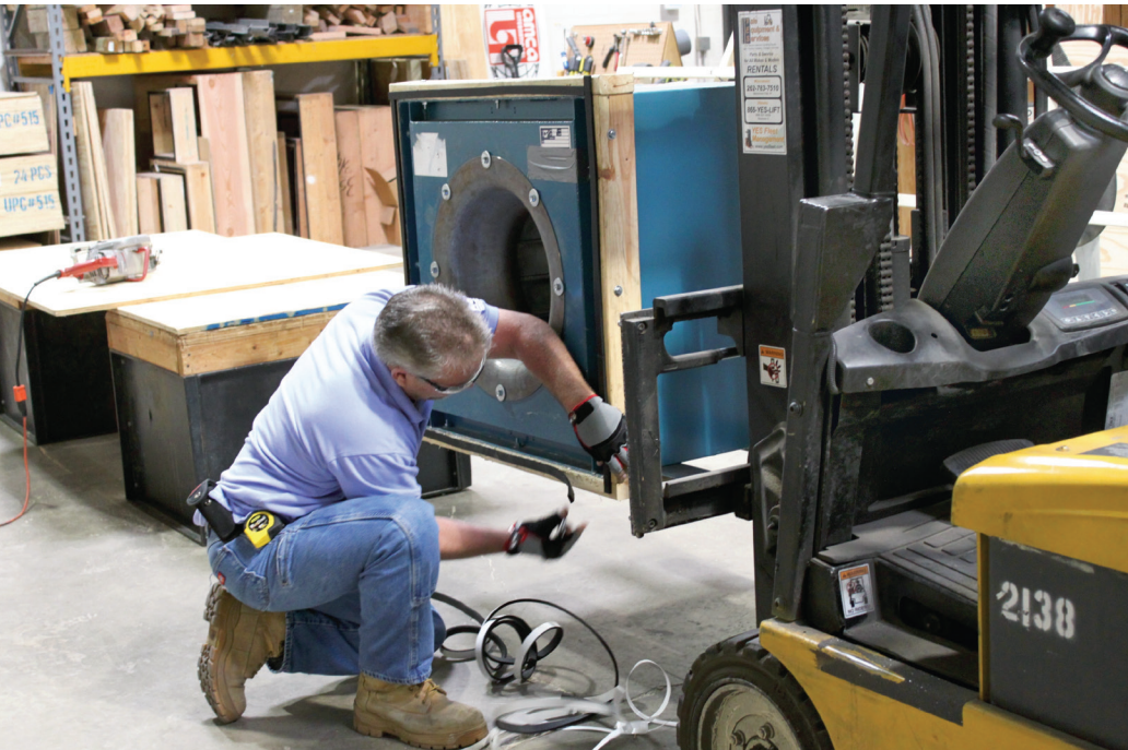
A fan is prepared for testing in the laboratory at AMCA International headquarters in Arlington Heights, Ill.
