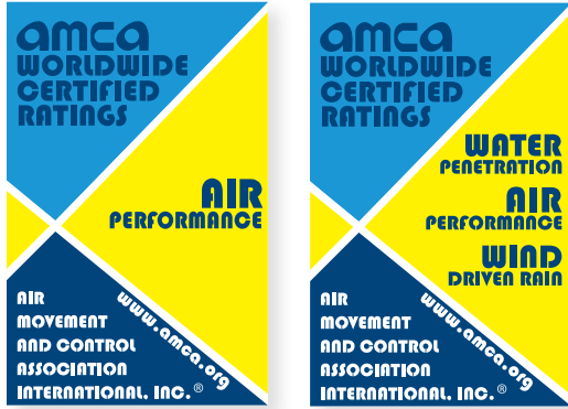
FIGURE 1. AMCA CRP seals for fans and dampers (left) and louvers (right). Note multiple certifications can be combined on one label.
