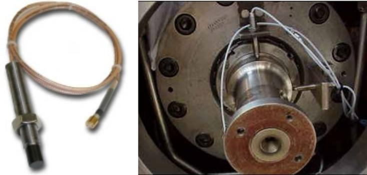
**Figure 13.** Eddy Current (Proximity) Probe
