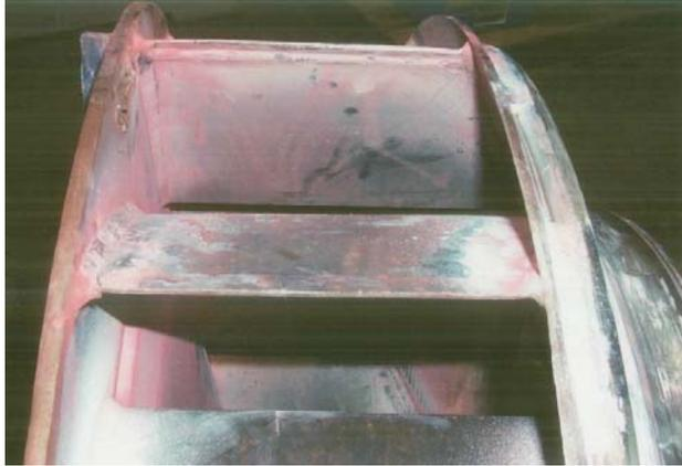
**Figure 23.** Impeller, Experimental Fatigue Test, Inspection Photo
