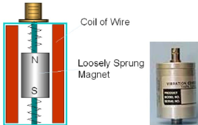
**Figure 11.** Velocity (“Seismic”) Transducer
