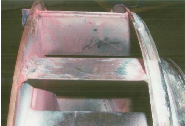
Figure 23. Impeller, Experimental Fatigue Test, Inspection Photo
