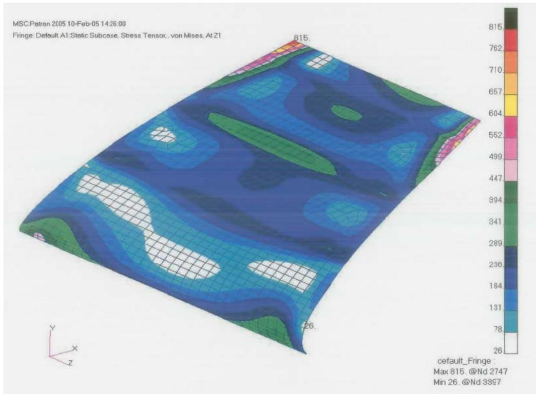
**Figure 26.** Finite Element Analysis Stress Plot of Airfoil
