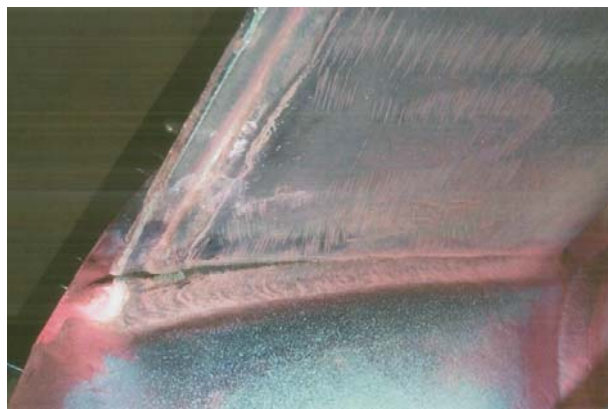
Figure 25. Impeller, Experimental Fatigue Test, Blade Crack Detail #2
