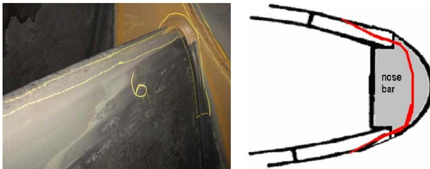
**Figure 20.** Airfoil Impeller Blade with Erosion
