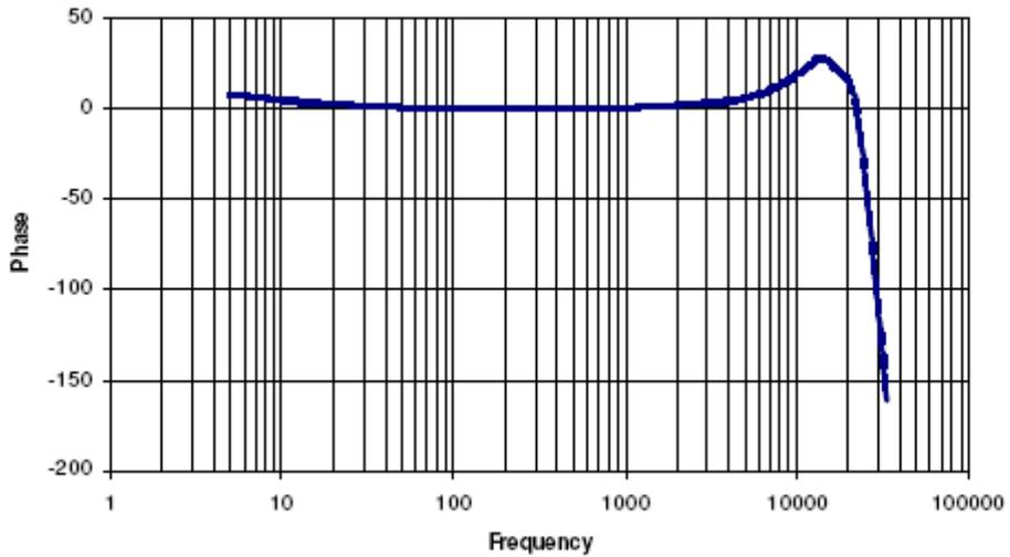
**Figure 9.** Accelerometer Phase Lag Roll-off vs. Frequency
