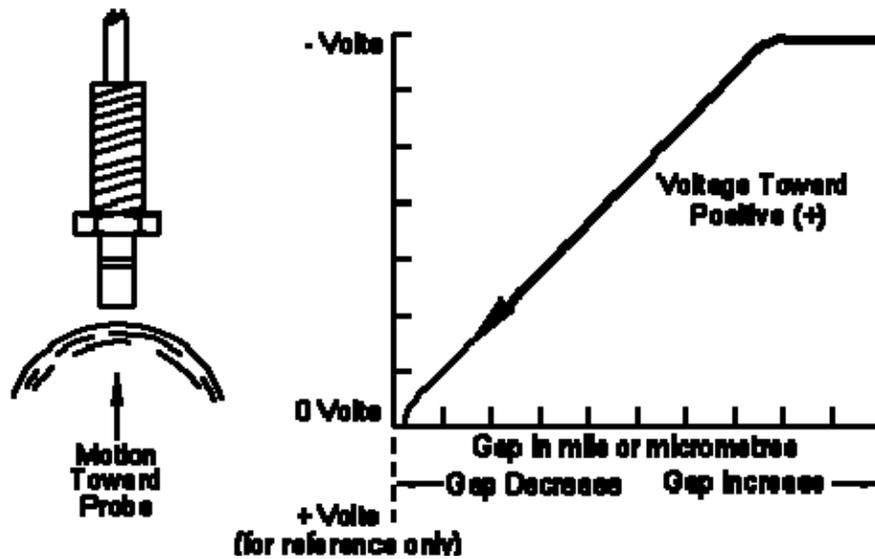
Figure 14. Proximity Probe Voltage vs. Gap Relationship
