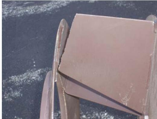
**Figure 19.** Cracked Impeller Blade
