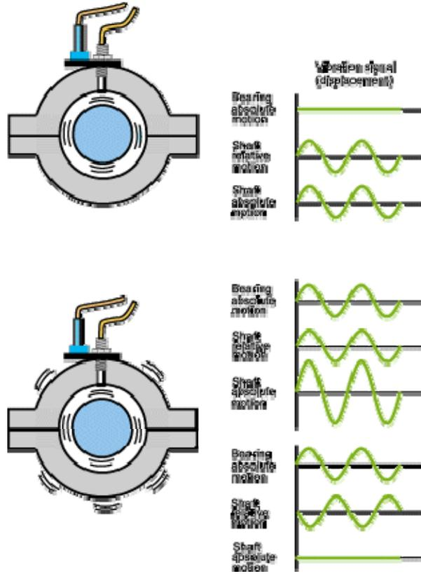
**Figure 15.** Vibration Transmissibility between Shaft and Bearing Casing
