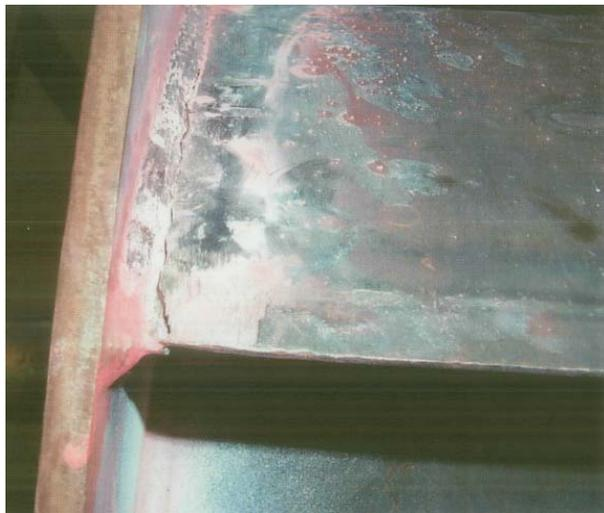
**Figure 24.** Impeller, Experimental Fatigue Test, Blade Crack Detail #1
