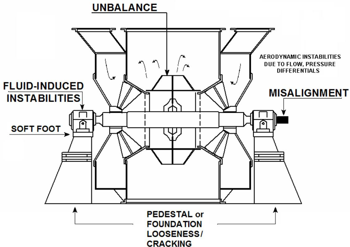
**Figure 18.** Fan Malfunctions
