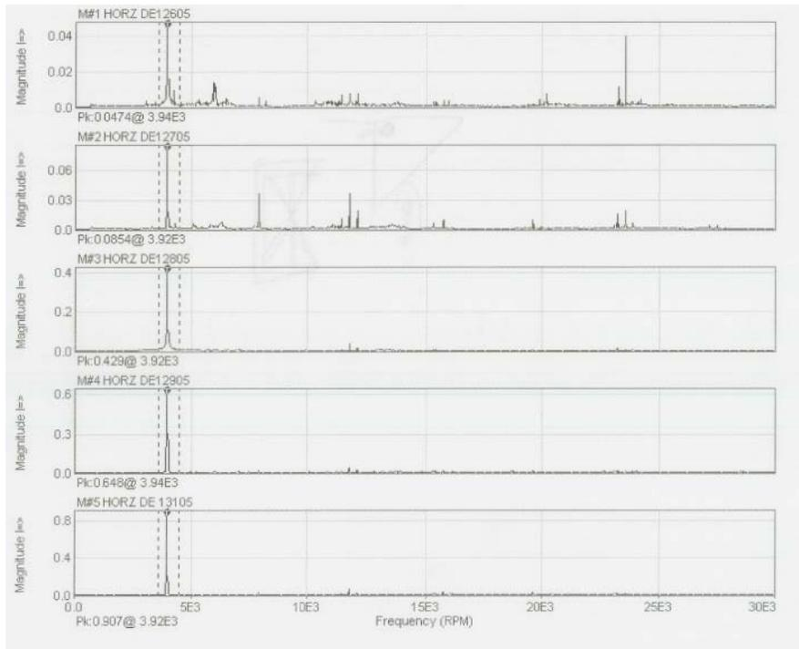
**Figure 22.** Drive End Vibration Spectrums [Accelerometer Mounted Horizontally]
