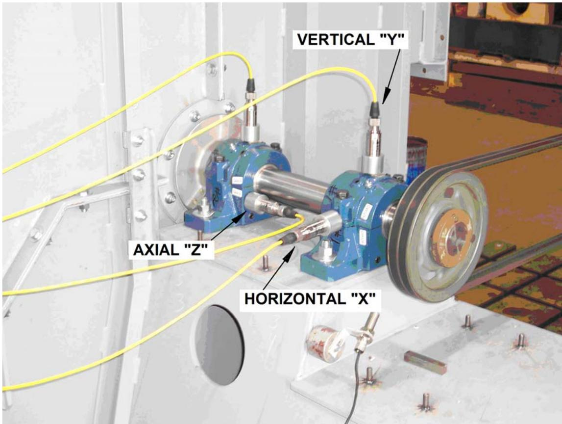
**Figure 5.** Vibration Measured in Three Different Planes
