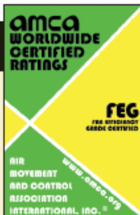
Figure 3: This sticker can be applied to fans bearing AMCA-certified ratings for fan efficiency grade, and it can also appear in literature and software programs in accordance with AMCA 211-2005 (rev 1-13) Certified Ratings Program - Product Rating Manual for Fan Air Performance.
