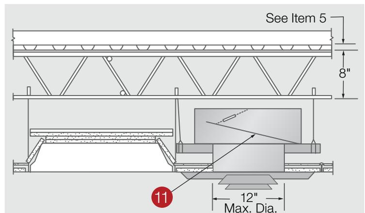
**11. Damper** — No. 13 MSG galv steel, 14 by 14 in. Protected on both surfaces with 1/16 in. ceramic fiber paper and held open with a Fusible Link. (Bearing the UL Listing Mark). Damper to overlap duct outlet 1 in. min.
