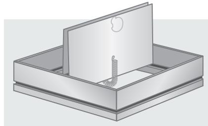
Figure 4. Example UL 555C-classified ceiling damper.
