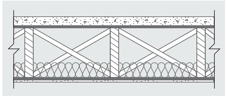
Figure 3. Example floor/ceiling assembly in which installation of ceiling dampers is prohibited.
