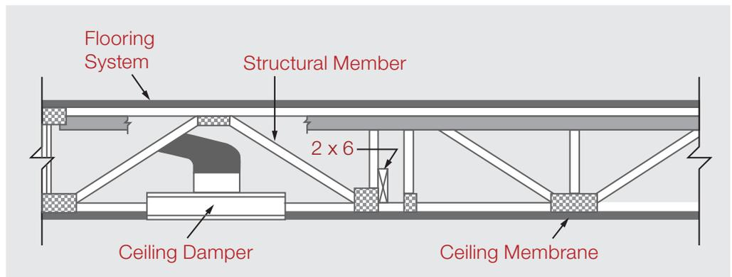
Figure 1. Example fire-rated floor/ceiling assembly.
