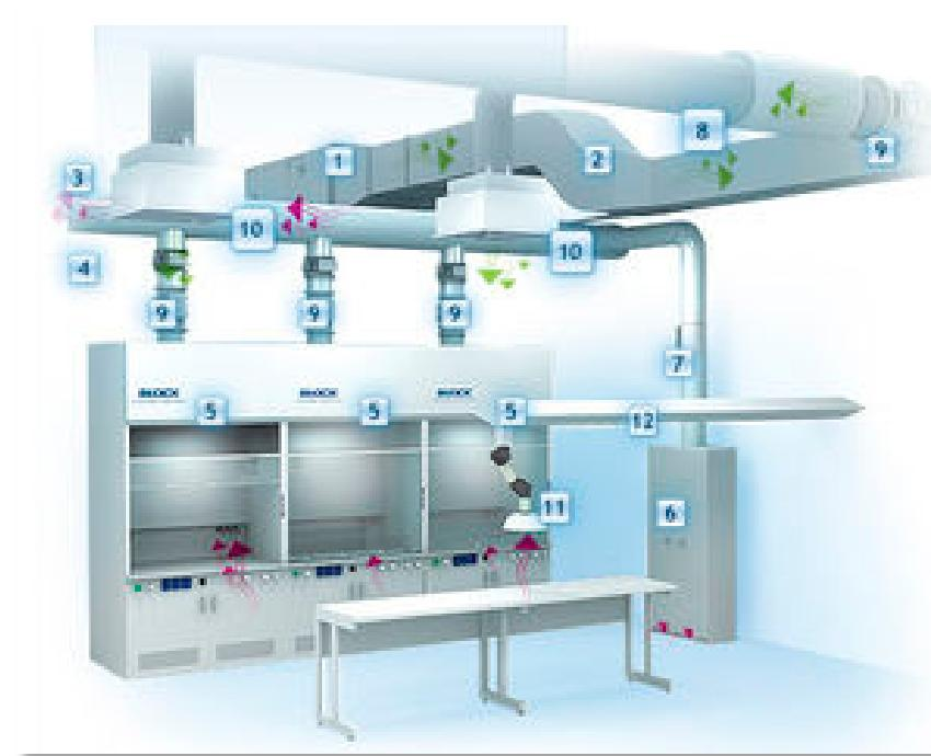
An exhaust system in which the total exhaust CFM varies depending on a number of conditions.
