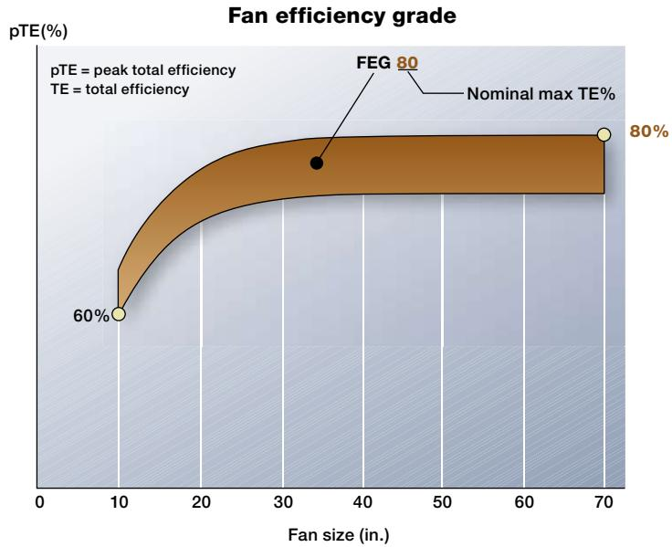
Figure 2: How a FEG is determined from a fan's peak total efficiency.
