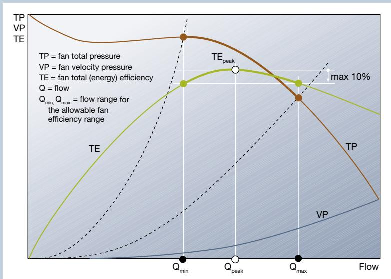
Figure 3: A typical fan performance curve, efficiency curve, and two system curves are shown. The system operating point should fall within a range around the peak efficiency. This figure shows an efficiency range on either side of the peak efficiency, the corresponding point on the fan curve, and the two associated system curves. The system should be designed to operate between these two system curves.
